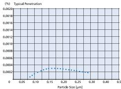
Esco cabinets use ULPA filters (per IEST-RP-CO01.3) instead of conventional HEPA filters commonly found in biological safety cabinets. While HEPA filters offer 99.99% typical efficiency at 0.3 micron level, ULPA filters provide >99.999% typical efficiency for particle sizes of 0.1 to 0.3 micron level.
