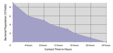
All exterior painted surfaces are powder-coated with Esco Isocide, an antimicrobial inhibitor to diminish contamination. Isocide is integrated into the coating substrate and cannot wash out or diminished by repeated cleaning. Performance results are available upon request. Contact Esco or your Esco Sales Representative for details.
